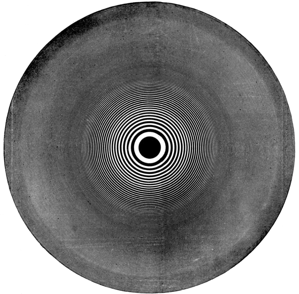
PLATE 2. ZONE-PLATE, FROM A DRAWING.
